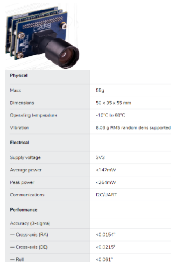
Fig. 3.21. CubeStar star tracker by CubeSpace [21]
